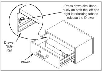
Figure 4. Removing Drawer
